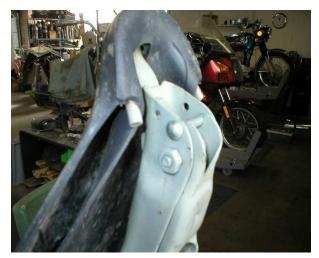
Once you have the nose piece correctly positioned; place the seat cover with nose piece installed into a shallow pan of very hot water. Just under boiling is best.. Wait about three minutes then remove the seat from the hot water and fit to the frame in the jig. Tighten the two carriage bolts which secure the nose piece to the seat frame. Position the bracket so that it looks centered and even.
