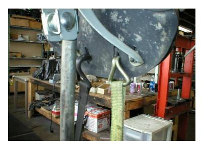
When you are sure that the nose is tight. Then you can evenly tension the two tie-down straps. The studs welded to the rear seat stretcher frame will pop into their respective holes in the seat frame after sufficient tension has been applied to both straps. Immediately install two new nuts and washers to the studs and tighten. Then release the tiedown straps, and you're DONE!
