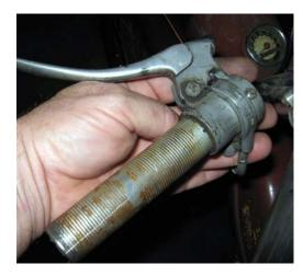
Step 5: Slide complete control assembly (Left side) off of the handlebar
