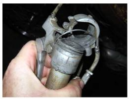
Step 6: Separate Gear Shift Control Housing from the rest of the assembly. Then remove old cable and discard.
