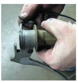
Step 8: Make sure that the cable is properly wrapped around the twist grip assembly.
