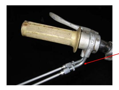
Step9: re-fit shift control assembly complete to handlebar. Pay special attention to position of short leg of cable (end with stepped end cap).
