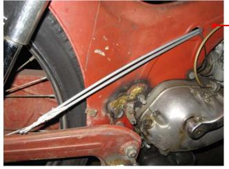
Step 10: Feed the cable through the moped body
